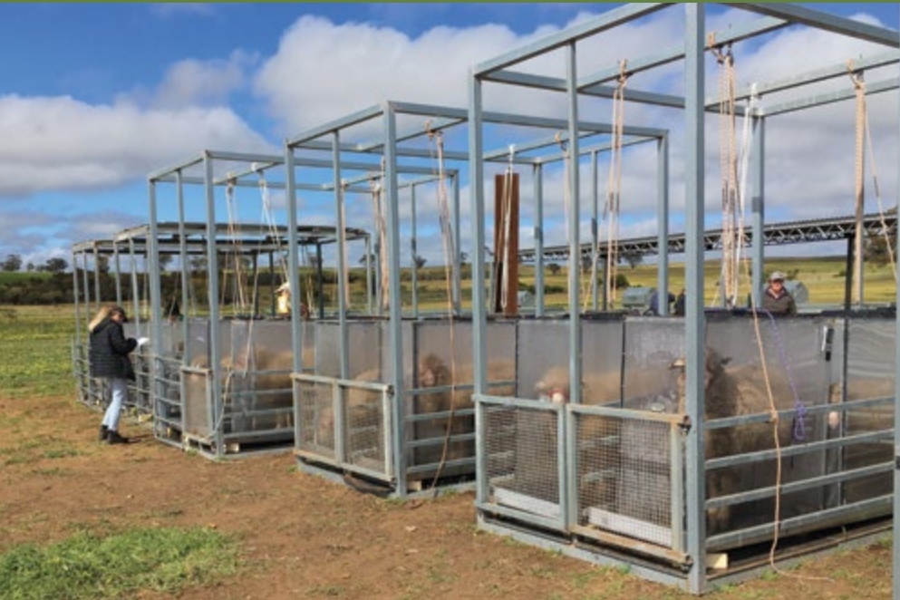
MLP F1 ewes being assessed for methane and carbon dioxide as a proxy for feed intake.
