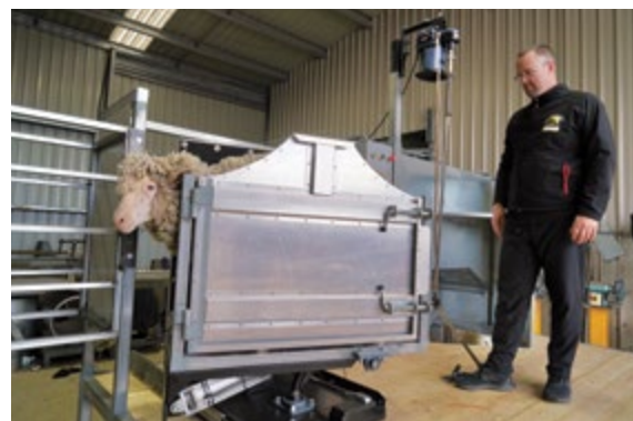
The pneumatically powered race section moving onto the board towards the shearer.
