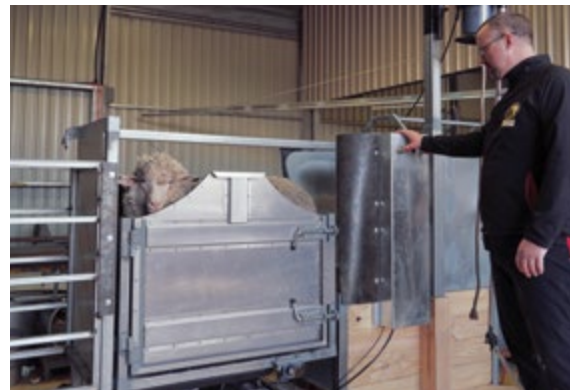
When ready for a sheep to be delivered, the shearer presses a button for the section containing a sheep to slide out towards him.
