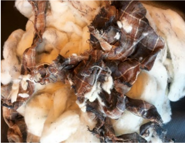
A shirt found in a processed batch (left) in China and the effect on the wool top (right).
