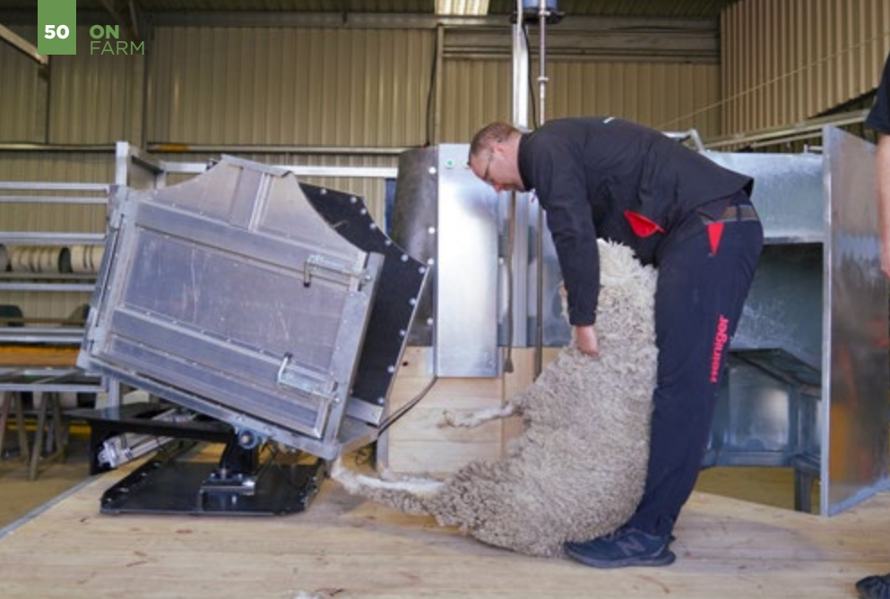
Shearer Josh Sneath with the prototype of the unit, showing how the sheep has been delivered directly to him, ready to start shearing. The empty unit is automatically returning to its position behind the board, for the next sheep.
