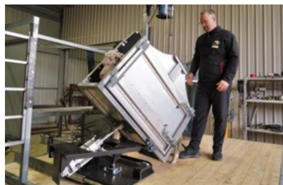
The section then gently tilts the sheep onto the board, into a position suitable for the shearer to hold it.
