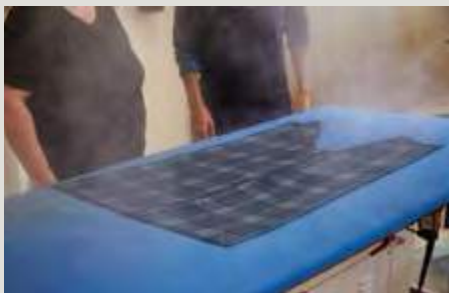
The heat vapour treatment that joins the two layers of knitwear.
